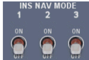
Picture. 4: INS Nav Mode Selector (for Triple INS configuration) with all switches in the OFF position
