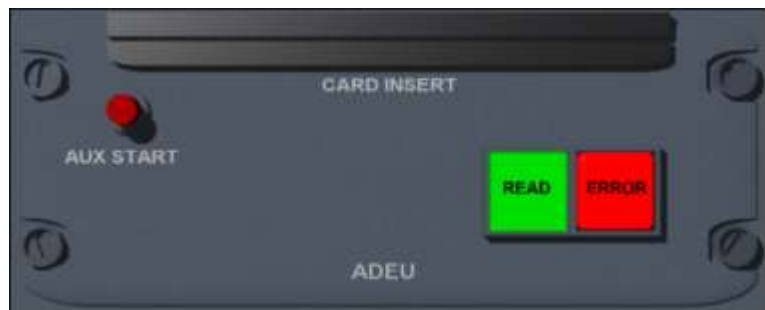
Picture .10: ADEU Control Panel
