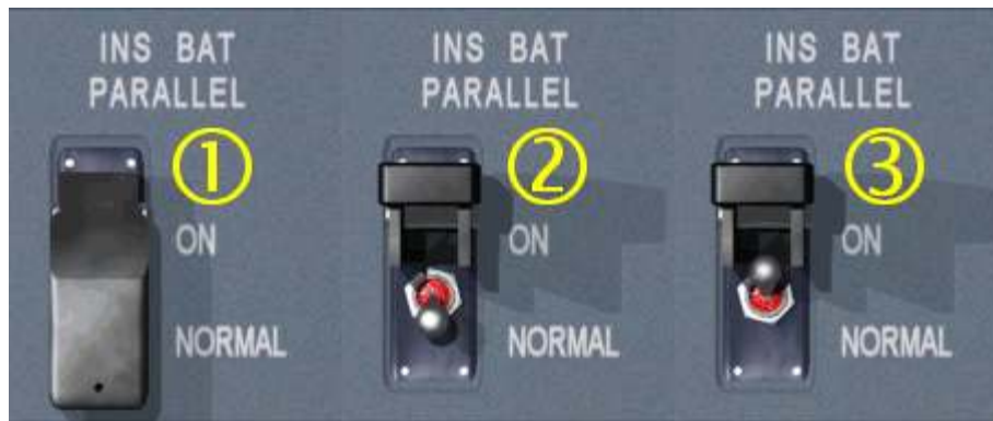
picture .3 :INS BAT PARALLEL Switch Positions
